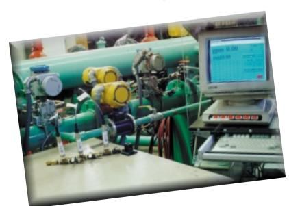
operator selects the type of assembly being tested, inputs the data on the assembly such as make model, etc. The size and orientation of the pipe is input and the system determines the correct calibration curve so that the corrected flow curve is generated automatically.
